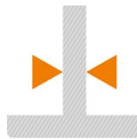
An unsupported wall is connected to other walls on less than 2 sides. Thinner walls may deform.
