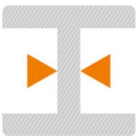
A supported wall is connected to other walls on two or more sides. Limit wall height to 10x wall thickness.
