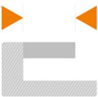
Longer unsupported horizontal overhangs may deform. Consider applying temporary supports.
