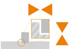
Parts for assembly should be designed with at least the recommended tolerance clearance.
