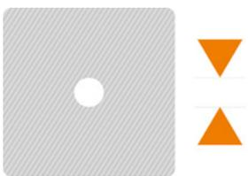
Smaller diameter holes may disappear/fill during print. Highly dependent on resin properties.
