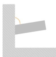
Larger angles may cause deformation. Consider applying temporary supports to overhangs.
