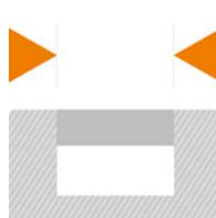
Longer bridge spans may deform. Try to avoid using (wide) bridges, or adjust the geometry if possible.
