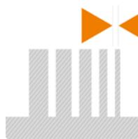
Limit the diameter:height ratio to 1:7.
